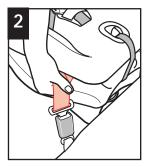
Grasp both vehicle belts together just behind the buckle plate and unbuckle. **NOTE**: If the buckle plate ends up behind the child restraint, grasp the belts to the outside of the child restraint, as close to the buckle plate as possible.
